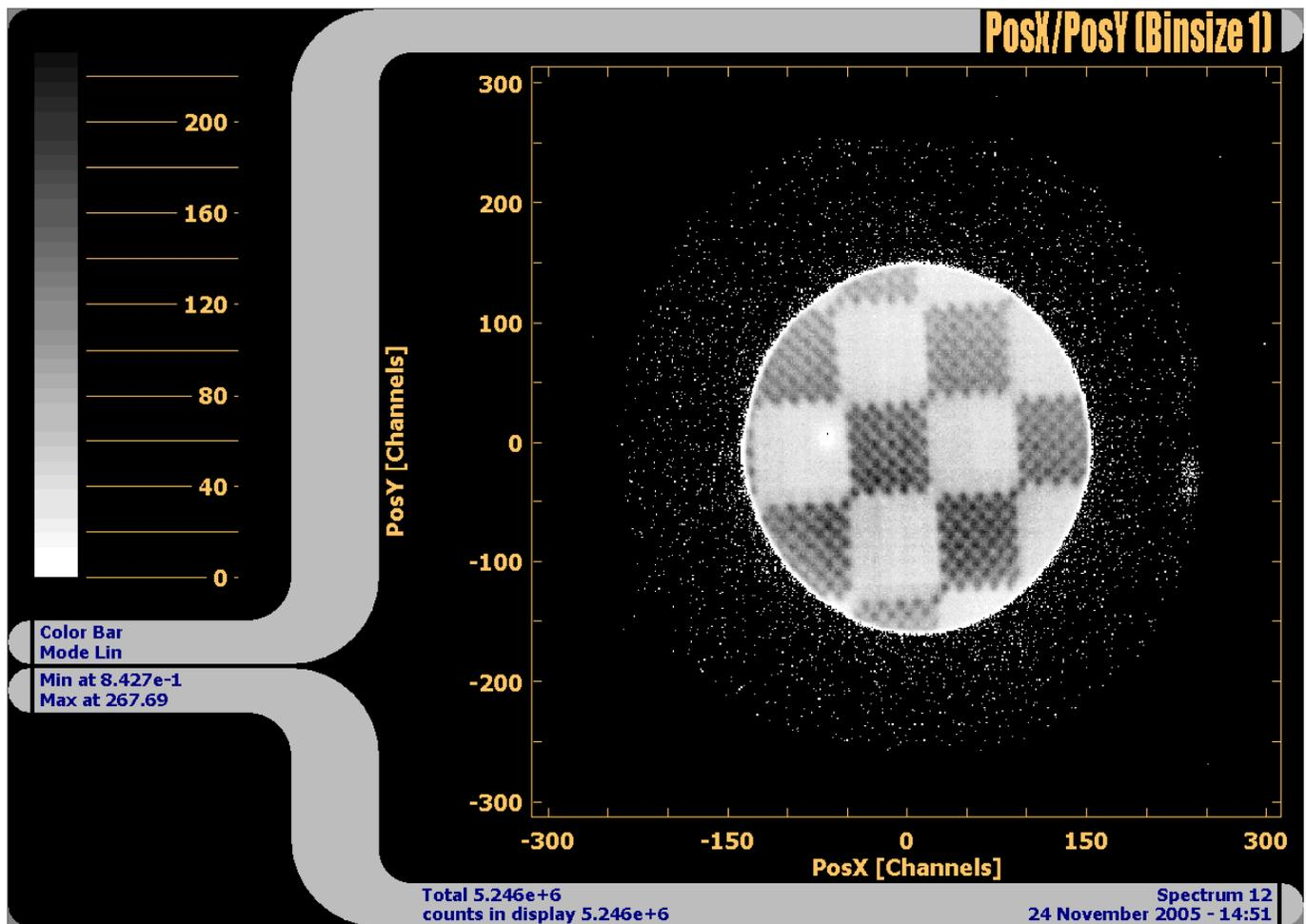
Figure 1: LEEM image taken from a micro-structured sample with a standard **DLD40**. Each white spot in the outer part of the image comes from individual dark counts of the microchannel plate (MCP).
