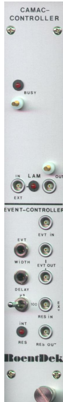
Figure 1.1: CCC1 Front Panel
