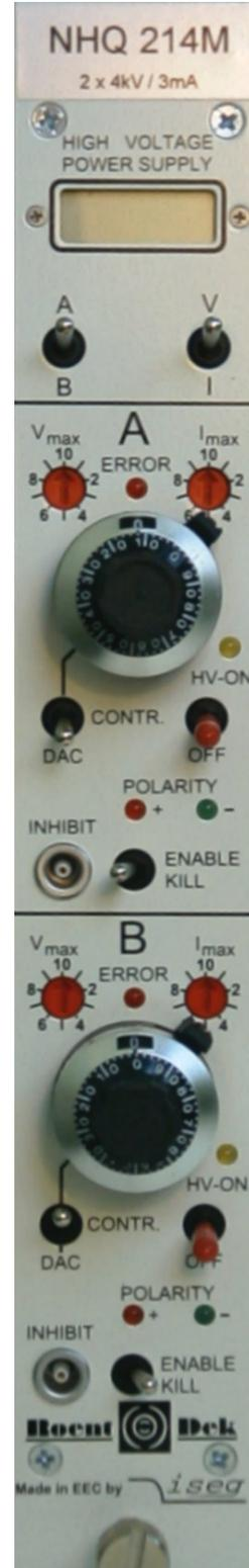
Figure: 2x4kV high-voltage power supply (front panel)
