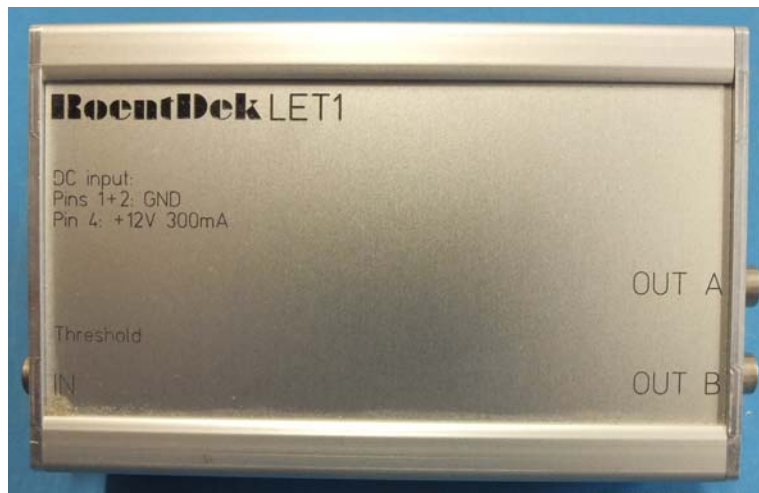
Figure: LET1 module. The LET1+version is similar but biased via an USB socket.
