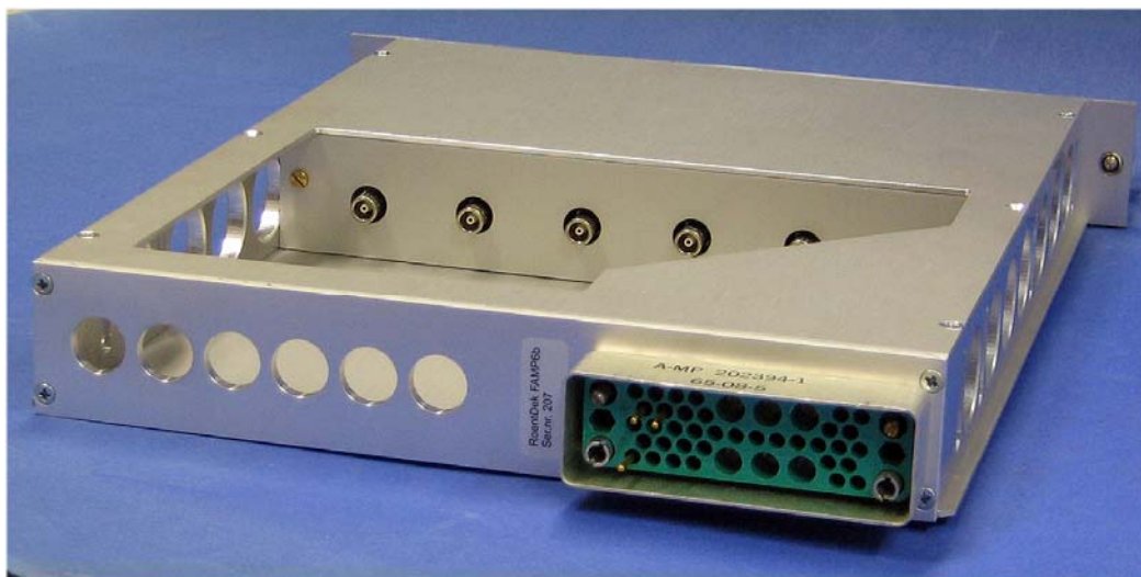
Figure 1: rear panel of FAMP6 (top) with NIM connector and signal inputs, right: front panel of FAMP6 with signal outputs.
