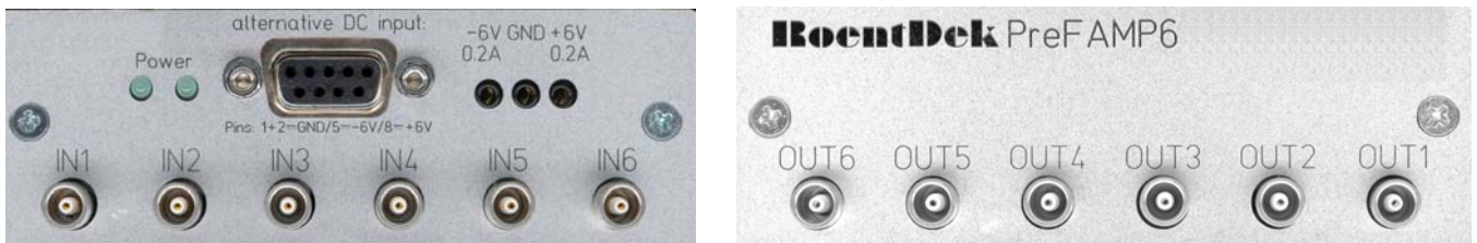
Figure 4: rear panel of PreFAMP6 (left) with signal inputs and DC power input via 9-pin sub-D connector or 2mm pins. Right: front panel of PreFAMP6 with signal outputs.
