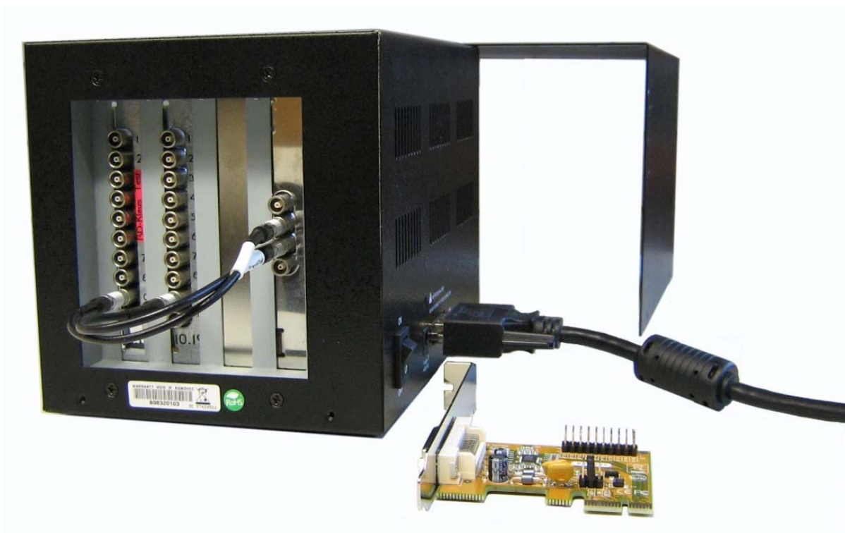
PCI2PCIe crate, here with two TDC8HP boards and clock card inserted. A PCIe adapter card and cable connection is shown on the lower right side. Not shown is the mains adapter (12V 3A) with cable.
